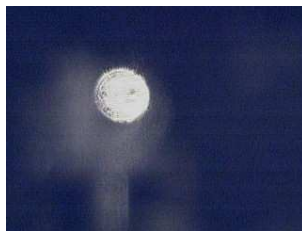
Figure 3.10: The light of the BAL converted in the Gaussian TEM_{00} mode of the Ti:Sa
